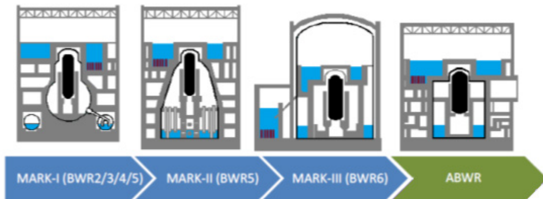
Figure 28.3-6 : Evolution of BWR SFP location
